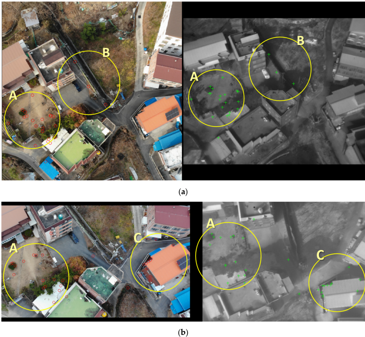
Figure 9. Understanding the characteristics of feature points of the building type: (a) visible nadir-looking vs. TIR oblique case; (b) visible oblique vs. TIR nadir-looking case.
