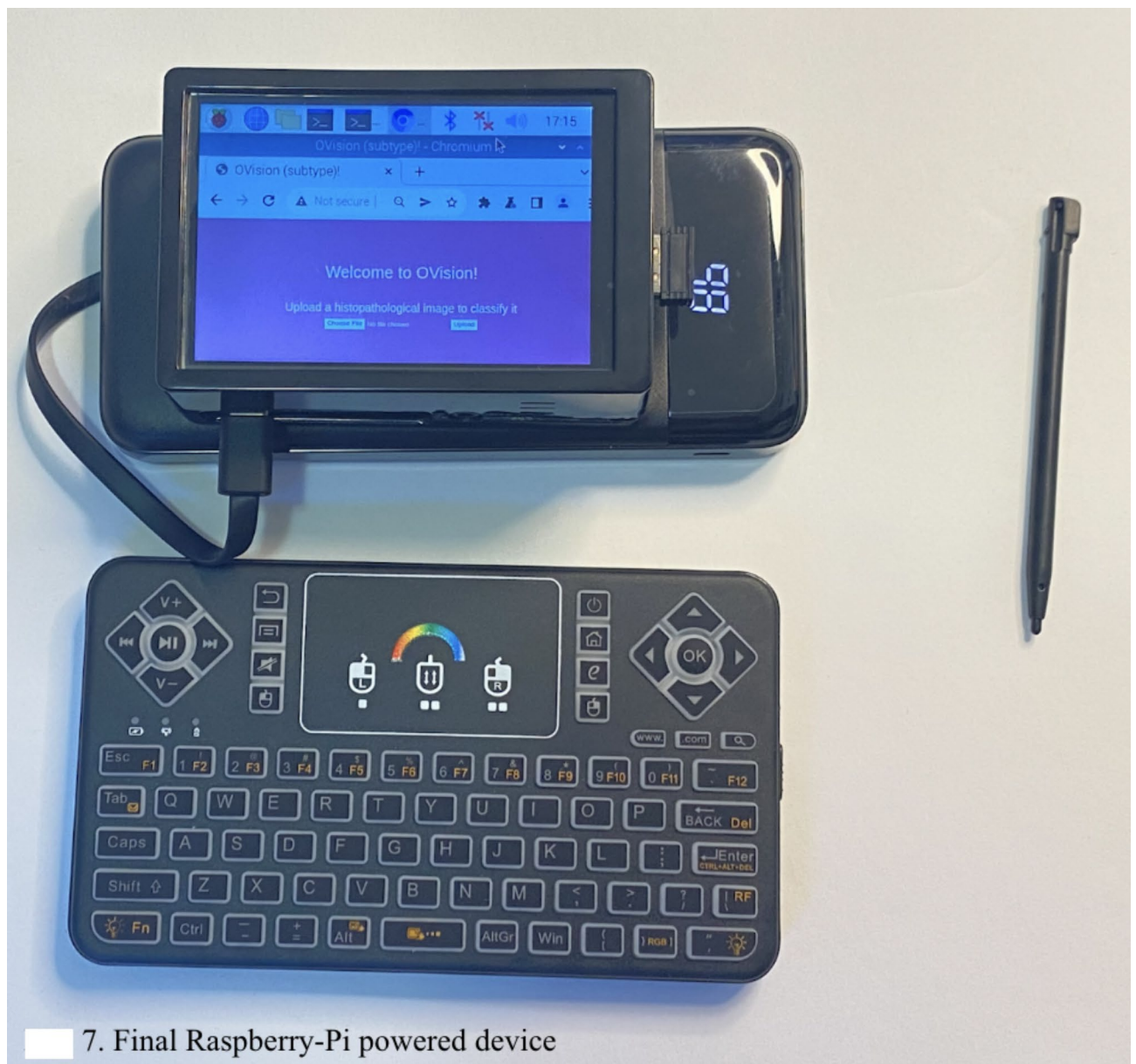
Fig. 6. Final Medical Device Framework - RaspberryPi powered compact (2.5 inch by 3 inch) final medical device with LCD, battery pack and optional mini keyboard. The final trained and validated model has been uploaded to the device and device is configured ready to accept image from USB drive and classify providing fast and accurate results in matter of seconds.
