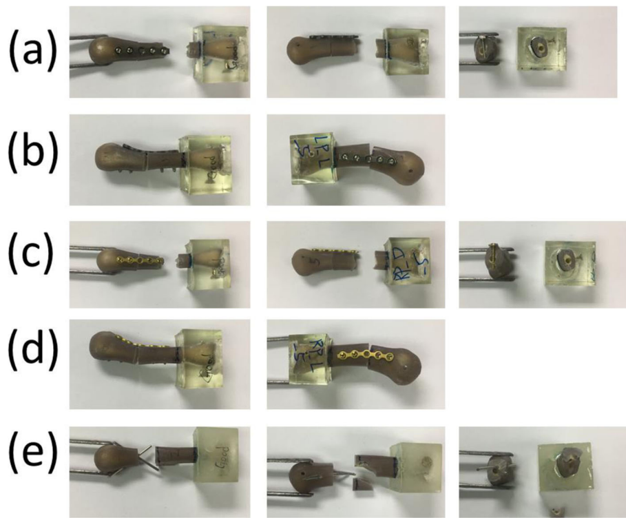
Fig. 5 Failure modes of the five fixation approaches: (a) locking plate with four locking bicortical screws on the dorsal side; (b) locking plate with four locking bicortical screws on the lateral side; (c) regular plate with four regular bicortical screws on the dorsal side; (d) regular plate with four regular bicortical screws on the lateral side; and (e) two K-wires. Left column, anterior–posterior view; middle column, lateral view; right column, cross-section view
