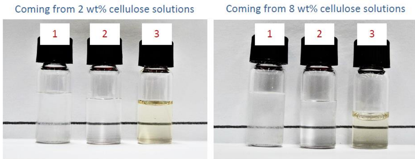
Figure 1. Picture of the supernatant phase obtained after addition of H 2 O at 20 °C (1), H 2 O at 4–5 °C (2), or AcOH at either 20 or 60 °C (3) to EMIMCl solutions with 2 wt% (left) and 8 wt% (right) cellulose contents.
