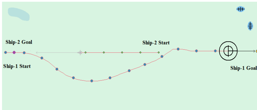
Figure 13. Verification result of ship trajectories in the head-on case.
