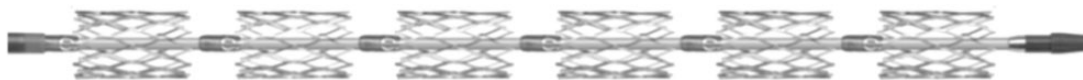
Figure 1. Illustration of the Multi-LOC stent delivery system. The Multiple Stent Delivery System with six self-expanding nitinol stents mounted on one central wire-guiding (0.035 inch) catheter is available in different versions with different stent diameters (from 5 to 8 mm) and two different working lengths (80 cm and 130 cm). The device represents a new generation of stent delivery technology, developed for provisional stenting of the femoropopliteal artery in case of insufficient results after balloon dilatation.
