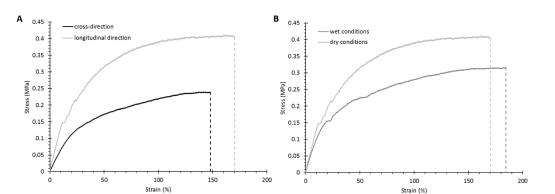
**Figure 5.** Stress–strain curves for KHC2000 scaffolds analyzed in different conditions: (**A**) in the cross-sectional and longitudinal directions in the dry state and at room temperature, and (**B**) in the longitudinal direction in wet and dry conditions at room temperature.
