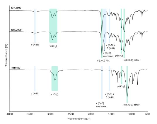
**Figure 2.** Attenuated Total Reflectance Fourier Transform Infrared (ATR-FTIR) spectra of KHC2000, NHC2000, and NHP407 poly(urethane)s. Light blue bars identify the characteristic peaks of newly formed urethane domains, and green bars refer to the typical bands of poly( $\varepsilon$ -caprolactone) (PCL) and P407.
