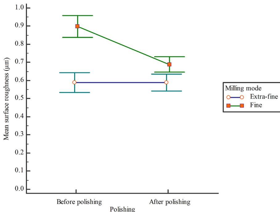
**Figure 5.** Mean surface roughness and standard error values (µm) before and after polishing in both milling modes.
