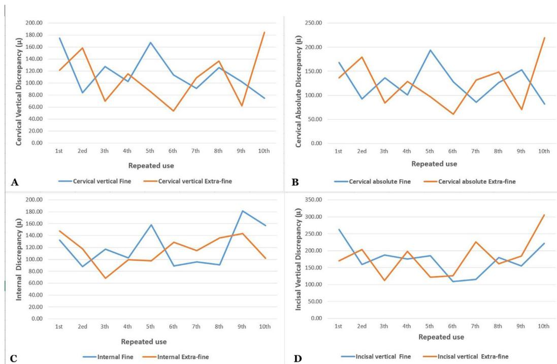
**Figure 6.** Discrepancy values ( $\mu$ ) in both milling modes during repeated use of the burs. A, cervical vertical discrepancy. B, cervical absolute discrepancy. C, internal discrepancy. D, incisal vertical discrepancy.
