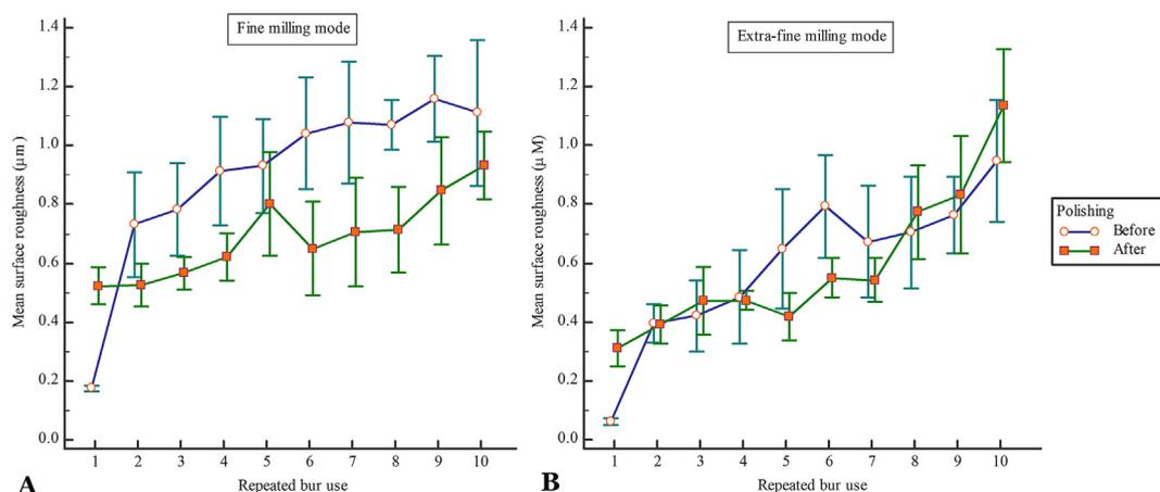
Figure 4. Mean surface roughness and standard error values ( $\mu\text{m}$ ) before and after polishing in both milling modes during repeated use of the burs. A, fine group. B, extra-fine group.
