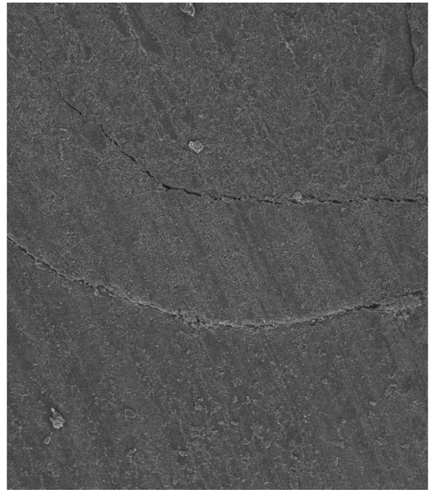
Figure 2. Field emission scanning electron microscope image analysis of a sectioned specimen at  $\times 200$  magnification.
