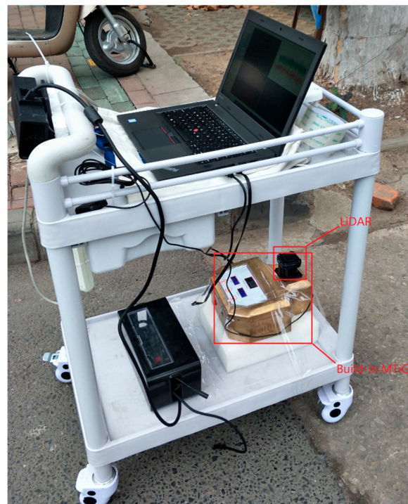
Figure 1. System hardware platform.
