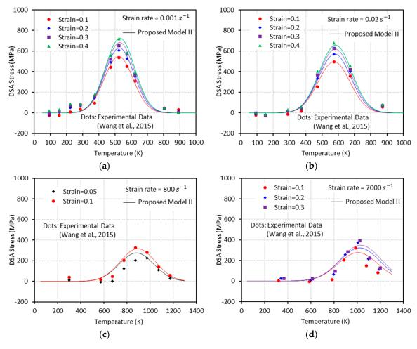
**Figure 13.** The DSA-induced flow stress versus temperature curves from the experiments [1] and the proposed model II with (a)  $\dot{\varepsilon} = 0.001 \, s^{-1}$ , (b)  $\dot{\varepsilon} = 0.02 \, s^{-1}$ , (c)  $\dot{\varepsilon} = 800 \, s^{-1}$ , and (d)  $\dot{\varepsilon} = 7000 \, s^{-1}$ .
