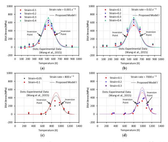
**Figure 8.** The DSA-induced flow stress versus temperature curves from the experiments [1] and the proposed model I with (**a**)  $\dot{\varepsilon} = 0.001 \, s^{-1}$ , (**b**)  $\dot{\varepsilon} = 0.02 \, s^{-1}$ , (**c**)  $\dot{\varepsilon} = 800 \, s^{-1}$ , and (**d**)  $\dot{\varepsilon} = 7000 \, s^{-1}$ .
