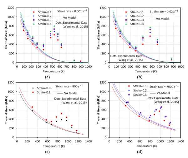
**Figure 5.** The thermal flow stress versus temperature curves from the experiments [1] and the VA model (Equation (15)) with (**a**)  $\dot{\varepsilon} = 0.001 \, s^{-1}$ , (**b**)  $\dot{\varepsilon} = 0.02 \, s^{-1}$ , (**c**)  $\dot{\varepsilon} = 800 \, s^{-1}$ , and (**d**)  $\dot{\varepsilon} = 7000 \, s^{-1}$ .
