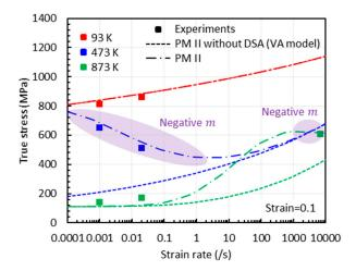
**Figure 25.** True stress versus strain rate graphs with three temperatures (93 K, 473 K, and 873 K) at  $\varepsilon = 0.1$ . The experimental data are from [1].
