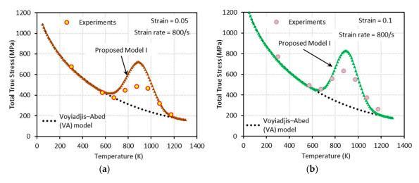
**Figure 11.** Comparisons between model predictions from the VA and proposed model I and experimental data from [1] on the total true stress versus temperature responses at (**a**)  $\varepsilon = 0.05$  and (**b**)  $\varepsilon = 0.1$ . Dynamic loading with  $\dot{\varepsilon} = 800 \, s^{-1}$  is applied.
