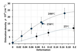
**Figure 2.** Dislocation density versus deformation graphs at different strain and temperature levels [12,13].
