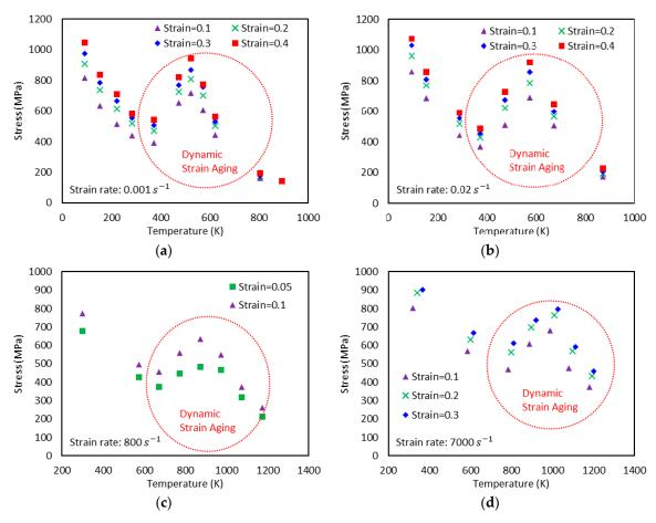
**Figure 1.** Experimental stress-temperature graphs for Q235B steel for different strain rates ( $\dot{\epsilon}$ ) and strain levels: (**a**)  $\dot{\epsilon} = 0.001 \, s^{-1}$ , (**b**)  $\dot{\epsilon} = 0.02 \, s^{-1}$ , (**c**)  $\dot{\epsilon} = 800 \, s^{-1}$ , and (**d**)  $\dot{\epsilon} = 7000 \, s^{-1}$  [1]. Dynamic strain aging (DSA) is observed in all cases.
