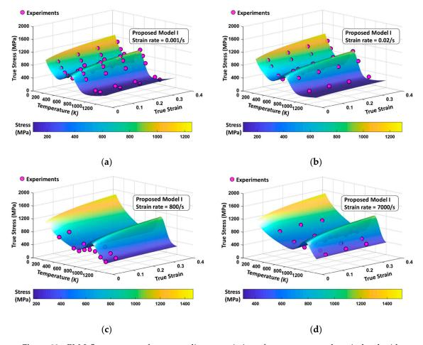
**Figure 23.** PM I flow stress surfaces according to variation of temperature and strain level with (a)  $\dot{\varepsilon} = 0.001 \, s^{-1}$ , (b)  $\dot{\varepsilon} = 0.02 \, s^{-1}$ , (c)  $\dot{\varepsilon} = 800 \, s^{-1}$ , and (d)  $\dot{\varepsilon} = 7000 \, s^{-1}$ . The experimental data are from [1].
