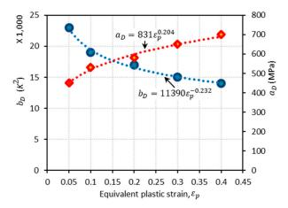
**Figure 6.** The plots of  $a_D$  and  $b_D$  versus  $\varepsilon_p$ . Dots for both of the parameters are obtained from the experimental data [1]. The corresponding trend lines are displayed using a power law form.
