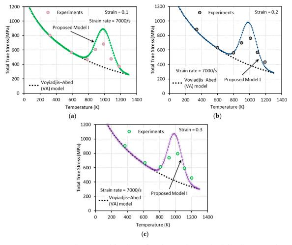
**Figure 12.** Comparisons between model predictions from the VA and proposed model I and experimental data from [1] on the total true stress versus temperature responses at (**a**)  $\varepsilon = 0.1$ , (**b**)  $\varepsilon = 0.2$ , and (**c**)  $\varepsilon = 0.3$ . Dynamic loading with  $\dot{\varepsilon} = 7000 \ s^{-1}$  is applied.
