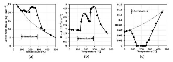
**Figure 3.** Profiles of model predictions (lines) and experimental data (dots) according to the temperature variation: (a) lower yield stress, (b) U - A and (c)  $\Omega$  [13].
