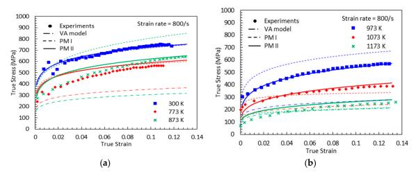
**Figure 21.** True stress-true strain curves from experimental measurement [1], predictions by the VA model, PM I, and PM II with  $\dot{\varepsilon} = 800 \, s^{-1}$ : (a) T = 300, 773 and 873 K (b) T = 973, 1073 and 1173 K.
