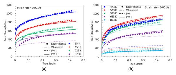
**Figure 19.** True stress-true strain curves from experimental measurement [1], predictions by the VA model, proposed model (PM) I, and PM II with  $\dot{\varepsilon} = 0.001 \ s^{-1}$ : (a) T = 93, 153, 223 and 373 K (b) T = 473, 523, 573, 623 and 893 K.
