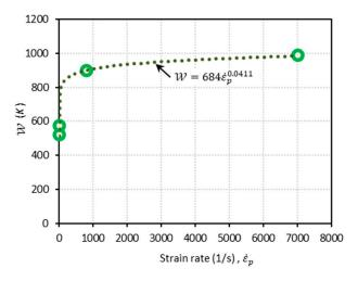
**Figure 7.** The plot of W versus  $\dot{\varepsilon}_p$ . Dots for both of the parameters are obtained from the experimental data [1]. The corresponding trend lines are displayed using a power law form.
