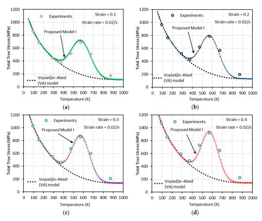
**Figure 10.** Comparisons between model predictions from the VA and proposed model I and experimental data from [1] on the total true stress versus temperature responses at (a)  $\varepsilon = 0.1$ , (b)  $\varepsilon = 0.2$ , (c)  $\varepsilon = 0.3$ . and (d)  $\varepsilon = 0.4$ . Quasi-static loading with  $\dot{\varepsilon} = 0.02 \, s^{-1}$  is applied.
