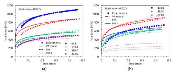
**Figure 20.** True stress-true strain curves from experimental measurement [1], predictions by the VA model, PM I, and PM II with  $\dot{\varepsilon} = 0.02 \ s^{-1}$ : (a) T = 93, 153, 289 and 373 K (b) T = 473, 573 and 673 K.
