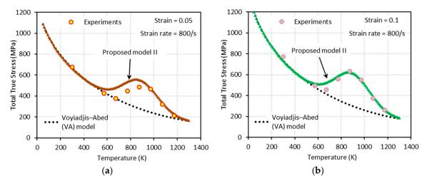
**Figure 16.** Comparisons between model predictions from the VA and proposed model II and experimental data from [1] on the total true stress versus temperature responses at (a)  $\varepsilon = 0.05$  and (b)  $\varepsilon = 0.1$ . Dynamic loading with  $\dot{\varepsilon} = 800 \, s^{-1}$  is applied.
