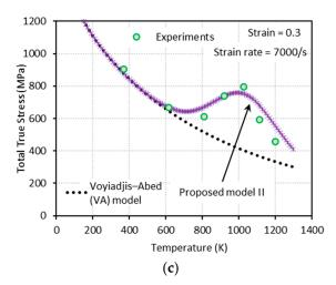
**Figure 17.** Comparisons between model predictions from the VA and proposed model II and experimental data from [1] on the total true stress versus temperature responses at (a)  $\varepsilon = 0.1$ , (b)  $\varepsilon = 0.2$ , and (c)  $\varepsilon = 0.3$ . Dynamic loading with  $\dot{\varepsilon} = 7000 \, s^{-1}$  is applied.
