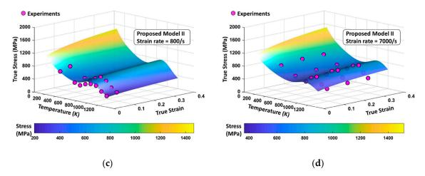
**Figure 24.** The PM II flow stress surfaces according to variation of temperature and strain level with (a)  $\dot{\varepsilon} = 0.001 \ s^{-1}$ , (b)  $\dot{\varepsilon} = 0.02 \ s^{-1}$ , (c)  $\dot{\varepsilon} = 800 \ s^{-1}$ , and (d)  $\dot{\varepsilon} = 7000 \ s^{-1}$ . The experimental data are from [1].
