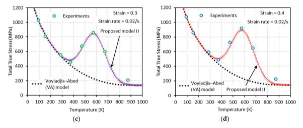
**Figure 15.** Comparisons between model predictions from the VA and proposed model II and experimental data from [1] on the total true stress versus temperature responses at (a)  $\varepsilon = 0.1$ , (b)  $\varepsilon = 0.2$ , (c)  $\varepsilon = 0.3$ , and (d)  $\varepsilon = 0.4$ . Quasi-static loading with  $\dot{\varepsilon} = 0.02 \, s^{-1}$  is applied.
