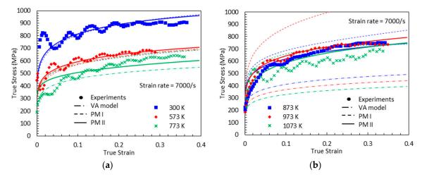
**Figure 22.** True stress-true strain curves from experimental measurement [1], predictions by the VA model, PM I, and PM II with  $\dot{\varepsilon} = 7000 \ s^{-1}$ : (a) T = 300, 573 and 773 K (b) T = 873, 973 and 1073 K.
