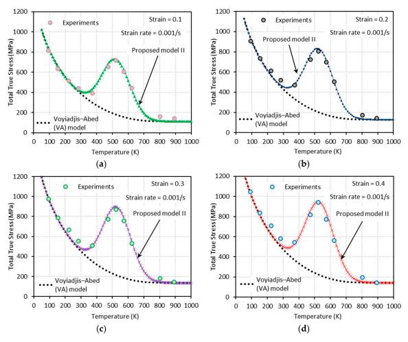
**Figure 14.** Comparisons between model predictions from the VA and proposed model II and experimental data from [1] on the total true stress versus temperature responses at (a)  $\varepsilon = 0.1$ , (b)  $\varepsilon = 0.2$ , (c)  $\varepsilon = 0.3$ , and (d)  $\varepsilon = 0.4$ . Quasi-static loading with  $\dot{\varepsilon} = 0.001 \, \text{s}^{-1}$  is applied.
