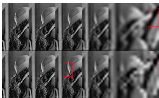
Figure 1. Accumulated reconstructions from each level of DTCWT ( top ) and DWT ( bottom ).
