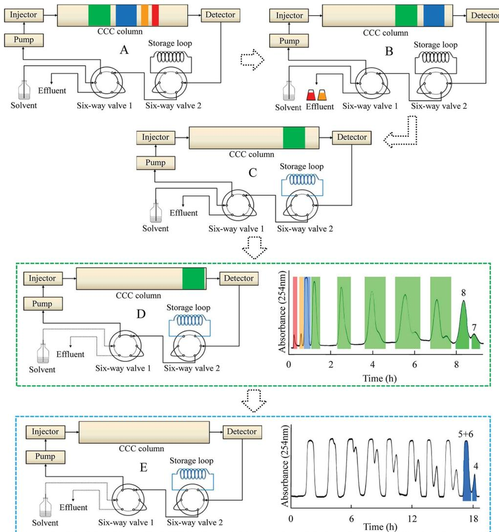
Fig. 4 Schematic diagram of online-storage inner-recycling CCC separation procedure. Solvent system: *n*-heptane/ethyl acetate/methanol/acetic acid (5 : 4 : 1 : 1, v/v); flow-rate: 2.0 mL min<sup>-1</sup>, detection wavelength: 254 nm. (A) Separation procedure, (B) separation of Fr. I and II in Fig. 3, (C) online-storage of Fr. III, (D) inner-recycling separation of Fr. IV, (E) inner-recycling separation of Fr. III.
