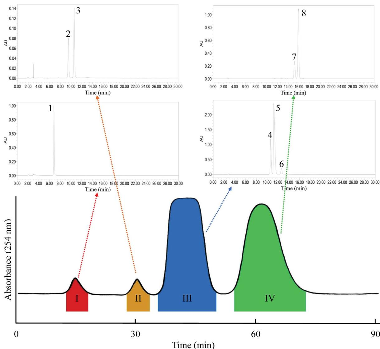
Fig. 3 HSCCC chromatogram of one-step separation mode. Solvent system: *n*-heptane/ethyl acetate/methanol/acetic acid (5 : 4 : 1 : 1, v/v); flow-rate: 2.0 mL min<sup>-1</sup>, detection wavelength: 254 nm.
