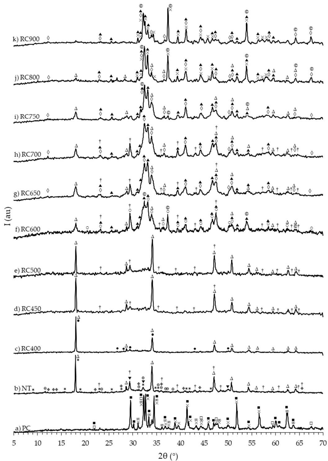
Figure 6. XRD analysis of PC, NT and RC. \Delta CH (portlandite); \dagger \text{CaCO}_3 (calcite); * \text{AF}_t (ettringite); \infty gypsum; \odot CaO; \blacksquare \text{C}_3\text{S} ; \bullet tobermorite 9\text{\AA} ; \blacktriangledown C-S-H; \times \beta\text{-C}_2\text{S} ; \blacktriangle \alpha'_L\text{-C}_2\text{S} ; \circ \text{C}_3\text{A} (calcium aluminum oxide); \square calcium aluminum iron oxide; \diamond \text{C}_4\text{AF} (brownmillerite); \Phi alumohydrocalcite; \theta calcium aluminum oxide carbonate hydrate.
