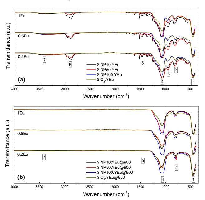
Figure 4. FT-IR spectra at room temperature of all SiNP: (a) before thermal treatment; and (b) after thermal treatment.
