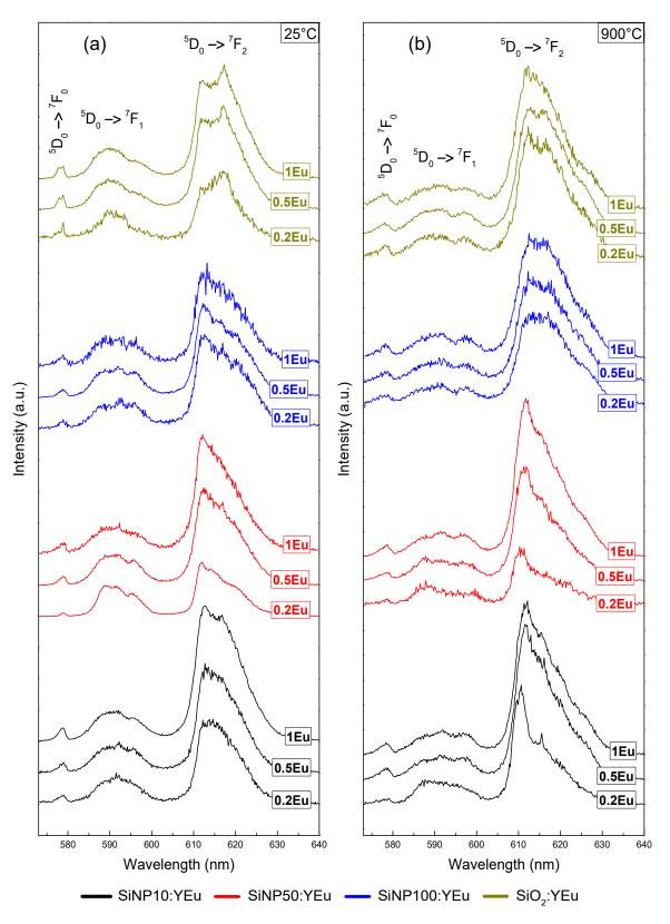
**Figure 5.** Emission spectra obtained under pulsed laser excitation at 532 nm at room temperature of Eu-doped silica nanoparticles and bulk (a) before and (b) after thermal treatment at 900  $^{\circ}$ C (the intensities are normalized to the maximum of the emission band  $^5D_0 \rightarrow ^7F_1$ ).
