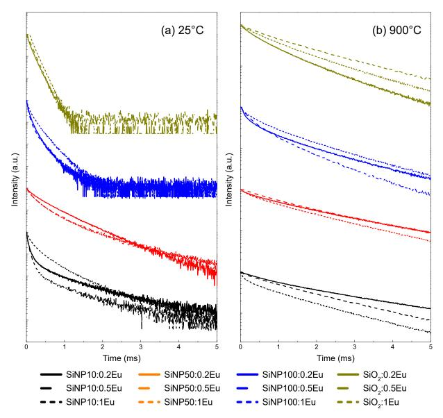
**Figure 6.** Luminescence decays of level  ${}^5D_0$  of Eu $^{3+}$  measured at the maximum intensity of the emission band  ${}^5D_0 \rightarrow {}^7F_2$  in Eu-doped silica nanoparticles and bulk: (a) before thermal treatment at 900 °C; and (b) after thermal treatment at 900 °C.
