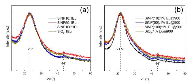
Figure 3. XRD patterns of SiNPX:1Eu and of bulk SiO<sub>2</sub>:1Eu: (a) before thermal treatment; and (b) after thermal treatment.
