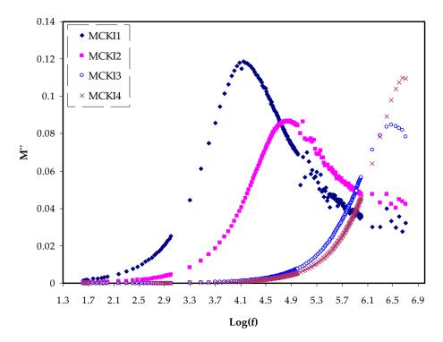
**Figure 7.** Electric modulus plot of  $M_i$  against log(f) for the MCKI samples.
