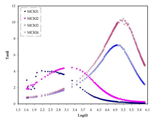
**Figure 5.** (*tan*  $\delta$ ) spectra versus frequency at room temperature for the MCKI electrolytes.
