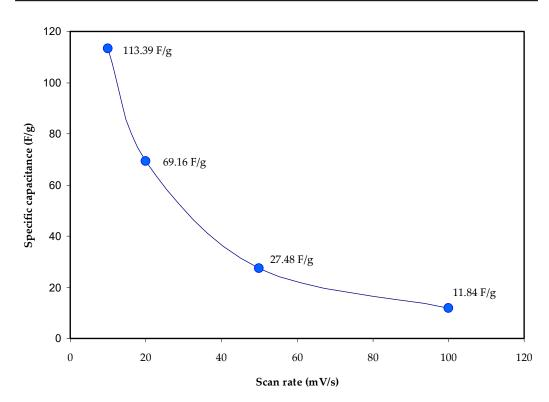
**Figure 12.** The calculated specific capacitance,  $C_s$  for the assembled EDLC at a different scan rate.
