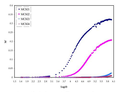
**Figure 6.** Electric modulus plot of  $M_r$  against log(f) for the MCKI samples.
