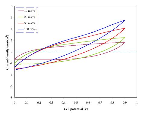
Figure 11. Cyclic voltammograms for the assemble EDLC in the potential range of 0 to 0.9 V.
