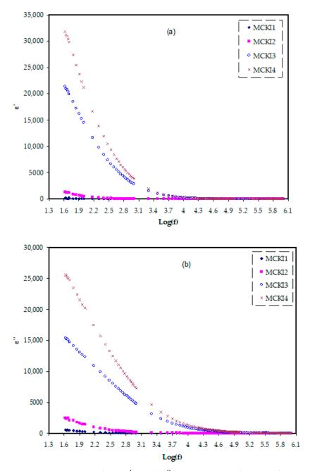
**Figure 4.** Dielectric plot for (a)  $\varepsilon'$  and (b)  $\varepsilon''$  variation against frequency for the MCKI samples.
