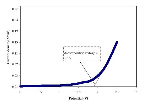
Figure 10. Current versus potential for the highest conducting (MCKI4) sample.
