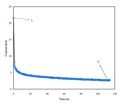
Figure 9. DC polarization curve of current versus time for the MCKI4 sample.
