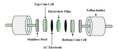
Figure 1. The schematic diagram of an EDLC cell. Adapted from reference [4].
