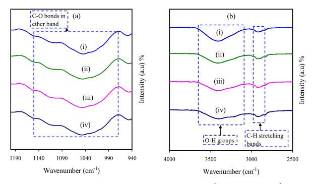
**Figure 8.** FTIR spectra of the MCKI samples at a wavenumber of (**a**) 940–1200 cm<sup>-1</sup> and (**b**) 2500–4000 cm<sup>-1</sup> for (i) MCKI1 (ii) MCKI2, (iii) MCKI3, and (iv) MCKI4 electrolyte samples.
