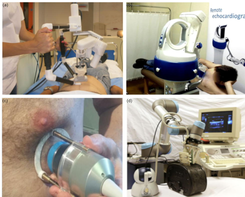
Fig. 1 Overview of different teleoperated robotic ultrasound systems. a MELODY system used in an abdominal exam (picture courtesy S. Avgousti, Cyprus University of Technology). b ReMeDi system used in a cardiac exam (figure by M. Giuliani et al. [21••] under CC-BY license). c TOURS system as utilized for remote exams on the International Space Station (reprinted from [23•], copyright [2018], with permission from Elsevier). d Teleoperated ultrasound platform with haptic device while acquiring an imaging phantom (figure by K. Mathiassen et al. [26] under CC-BY license)
