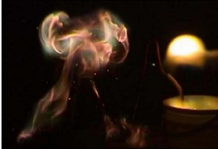
FIGURE 7. Two experimental fireballs in an erosive discharge by Emelin et al., one showing the streamers, the other a shell. From http://balllightning.narod.ru/hvewd.html , with kind permission.
