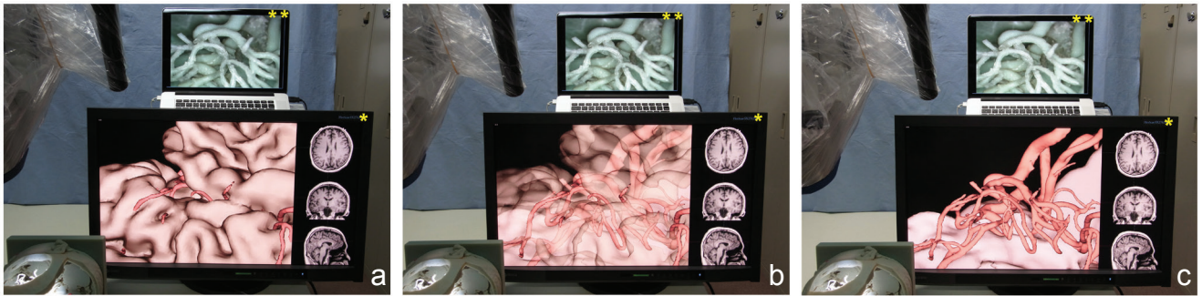
Fig. 4 The opacity of each structure in the 3D CG image could be changed on the monitor of the navigation system, revealing anatomical structures that were obstructed from view in the phantom model. a: Image before opacity was manipulated. b: Image after the opacity was changed to make the brain translucent. c: Image after the opacity was changed to make the brain transparent. CG: computer graphics, 3D: three-dimensional.
