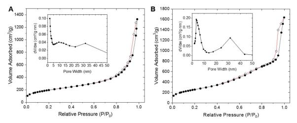
**Figure 2.** Adsorption-desorption isotherms at high relative pressures for the samples STMS50 (**A**) and WLMS80 (**B**) including Barrett–Joyner–Halenda (BJH) desorption pore volume plots for STMS50 (inset **A**) and WLMS80 (inset **B**).
