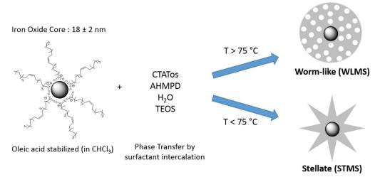
Scheme 2. Coating of IO NPs with stellate (STMS) or worm-like mesoporous silica (WLMS) morphologies.
