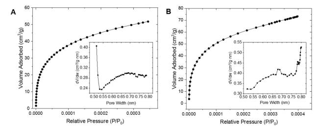
**Figure 3.** Adsorption isotherms at small relative pressures for STMS50 (**A**) and WLMS80 (**B**) including Horvarth–Kawazoe differential pore volume plots for STMS50 (inset **A**) and WLMS80 (inset **B**).
