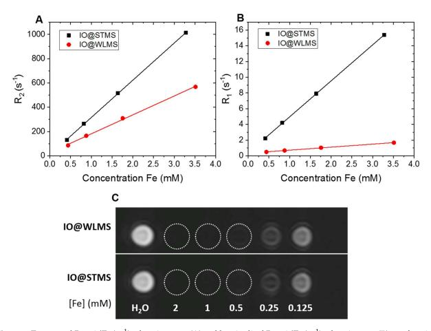
**Figure 5.** Transversal  $R_2 = 1/T_2$  (s<sup>-1</sup>) relaxation rates (**A**) and longitudinal  $R_1 = 1/T_1$  (s<sup>-1</sup>) relaxation rate (**B**) as a function of [Fe] (mM) for IO@STMS and IO@WLMS in water at 37 °C and 1.41 T; T<sub>2</sub>-weighted (**C**) MRI of IO@WLMS and IO@STMS, white, dotted-line circles indicate sample positions.
