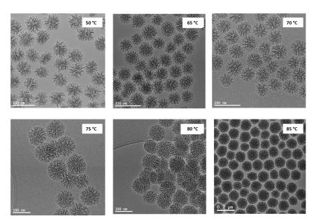
**Figure 1.** TEM images of MS NPs for different sol-gel reaction temperature:  $50 \,^{\circ}\text{C}$ ,  $65 \,^{\circ}\text{C}$ ,  $70 \,^{\circ}\text{C}$ ,  $75 \,^{\circ}\text{C}$ ,  $80 \,^{\circ}\text{C}$  and  $85 \,^{\circ}\text{C}$ . Below  $75 \,^{\circ}\text{C}$ , the MS present ST pore morphology whereas above  $80 \,^{\circ}\text{C}$ , WL type appears.
