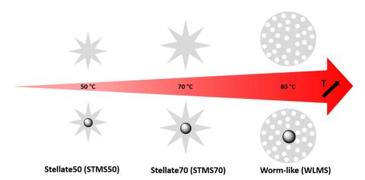
**Scheme 1.** Scheme illustrating the thermally controlled process to orient the pore morphology of mesoporous silica (MS) and IO@MS NPs from stellate (STMS) to worm like (WLMS).
