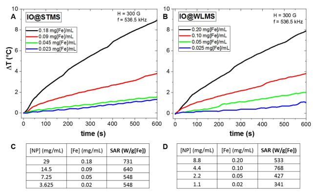
**Figure 6.** Temperature profiles as a function of time under alternating magnetic field (AMF) for different concentrations of IO@STMS (**A**) and IO@WLMS (**B**) including the corresponding SAR values for IO@STMS (**C**) and IO@WLMS (**D**).
