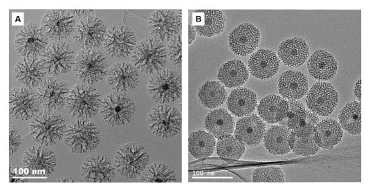
Figure 4. IO@STMS synthesized at 70 °C (A) and IO@WLMS synthesized at 80 °C (B).
