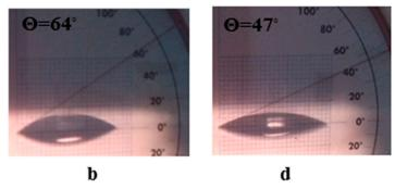
**Figure 5.** Optical images for water contact angle ( $\theta$ ) to glass surfaces that were uncoated (**a**) or coated by quercetin (Q) (**b**), titanium dioxide-decorated multi-walled carbon nanotubes (MWCNTs/TiO<sub>2</sub>) (**c**) quercetin quercetin titanium dioxide-decorated multi-walled carbon nanotubes nanocomposite (Q/MWCNTs/TiO<sub>2</sub>) (**d**).
