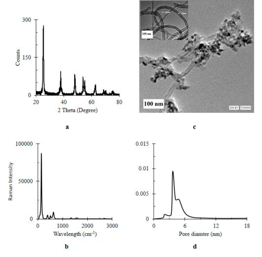
**Figure 1.** Characterization of titanium dioxide-decorated multi-walled carbon nanotubes (MWCNTs/TiO<sub>2</sub>) (a) XRD (X-Ray Diffraction) pattern; (b) Raman spectrum; (c) TEM (Transmission Electron Microscopy) image at a magnification bar of 100 nm (inset bare MCNTs); (d) pore diameter.
