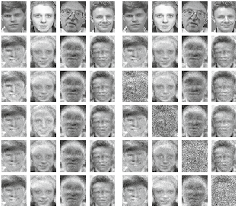
Fig. 6 Model inversion for a toy model trained on the AT&T Faces dataset with 4 classes. On the left side we show results for naive unlearning, on the right side for normalizing filtration . On either side: The top row shows one training image of each class, the second row reconstructions of classes by model inversion, the (i + 2) -th row shows the reconstructions after unlearning the class in the i -th column by the respective unlearning operation
