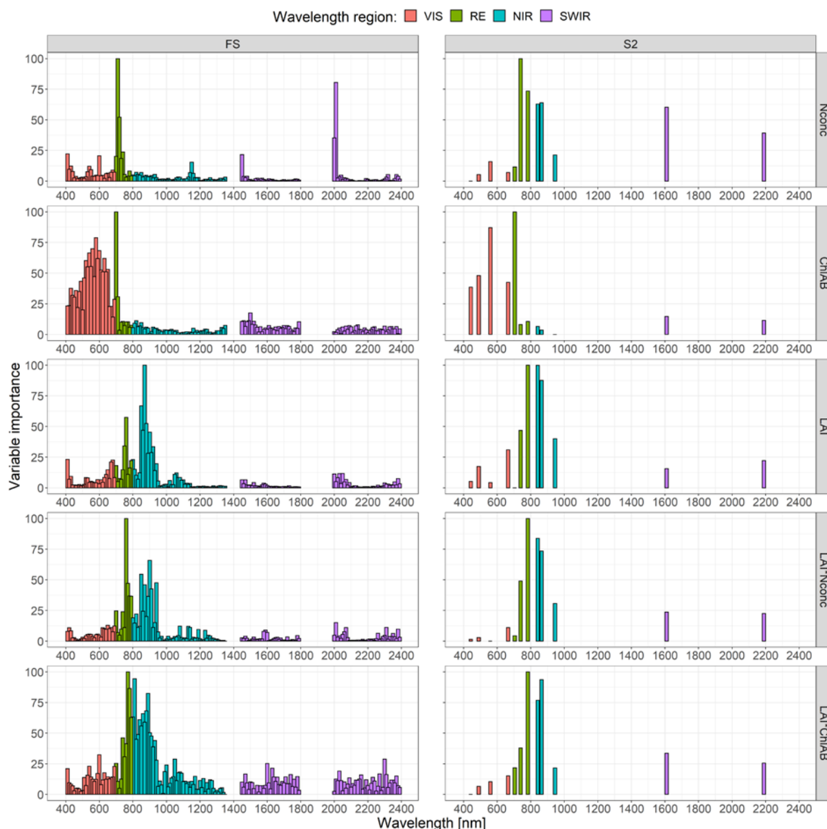
Figure 2. Calculated variable importance scores of the random forest regression (RFR) on the full dataset for the field spectrometer (FS, left) and the Sentinel-2 (S2, right) resampled data. The colors show the waveband regions visible (VIS: 400–690 nm), red edge (RE: 700–790 nm), near infrared (NIR: 800–1350 nm) and short-wave infrared (SWIR: 1450–2400 nm). The water absorption bands in the regions 1350–1450, 1790–1990 and >2400 nm were omitted due to their low signal to noise ratio.
