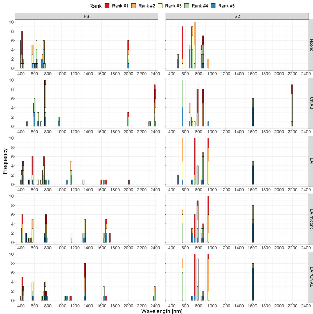
Figure 4. Occurrence of the top five ranked bands with lowest GPR sigma values for the ASD sensor ( left ) and the S2 resampled sensor ( right ). Data from 10-fold cross validation, e.g., 50 (10 folds \times 5 ranks) is the maximum possible occurrence.
