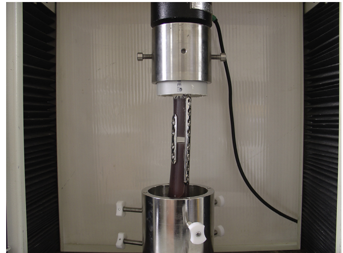
Fig. 2. Axial load was applied to the cylindrical potted end.
