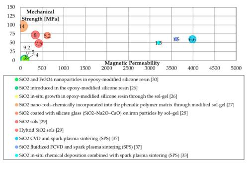
**Figure 1.** Magnetic (maximum permeability), mechanical (transverse rupture strength (TRS) [MPa]), and energetic properties (total iron losses 1 T@50 Hz [W/kg]) of SiO<sub>2</sub> coating processes.
