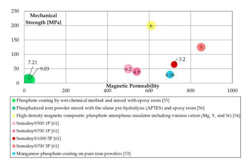
**Figure 3.** Magnetic (maximum permeability), mechanical (TRS [MPa]), and energetic properties (total iron losses 1 T@50 Hz [W/kg]) of phosphate coating processes.
