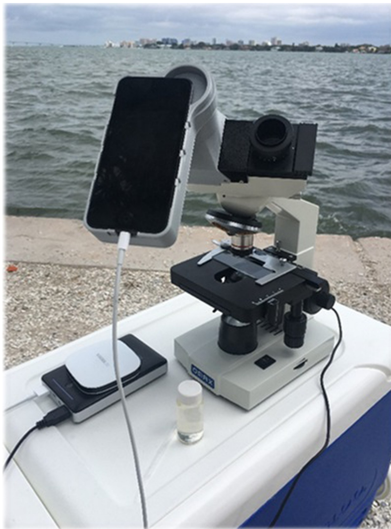
Fig 1. The HABscope setup. A photograph exhibiting the HABscope components, which are listed in Table 1 along with a list of suppliers and the 20 mL sampling vial.
