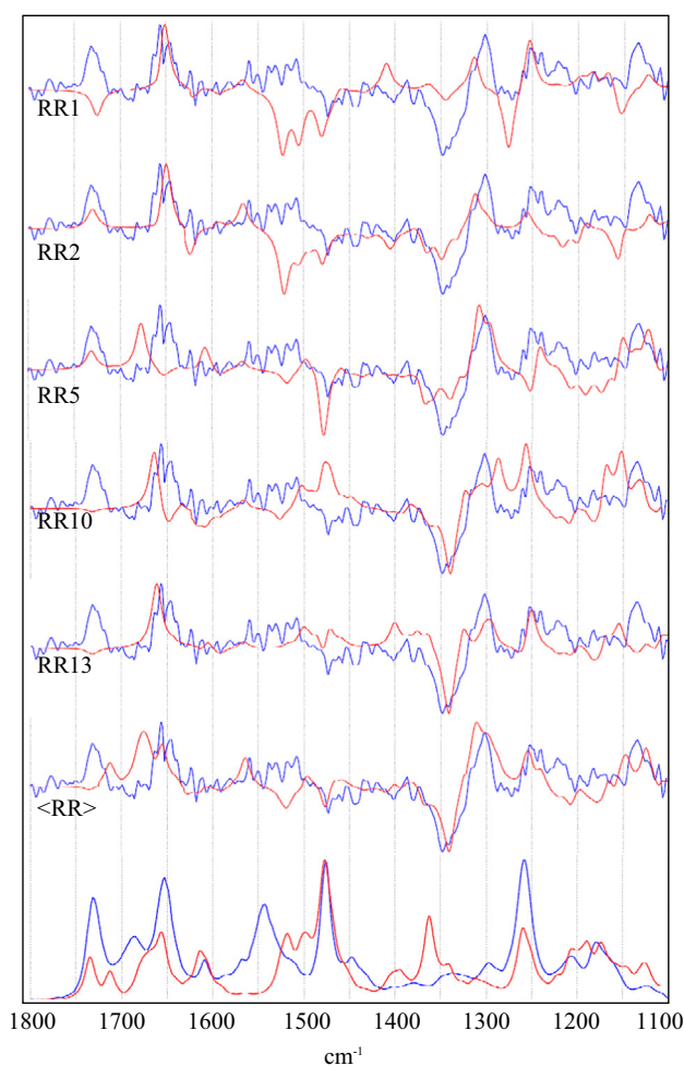
Fig. 4 The ligned VCD (top 6) and IR spectra of Otamixaban conformers with blue for the experiment and red for the calculation.
