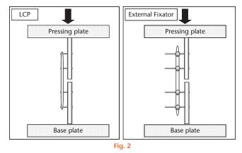
Diagram of constructs undergoing loading.
