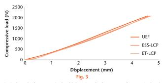
Typical graph of compressive load (N) against displacement at fracture site (mm) (ET-LCP, externalised titanium locking compression plate; ESS-LCP, externalised stainless steel locking compression plate; UEF, unilateral external fixator).
