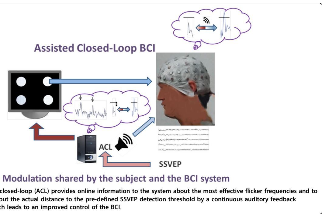
**Figure 1** The assisted closed-loop (ACL) provides online information to the system about the most effective flicker frequencies and to the human subject about the actual distance to the pre-defined SSVEP detection threshold by a continuous auditory feedback (speaker symbol), which leads to an improved control of the BCI.
