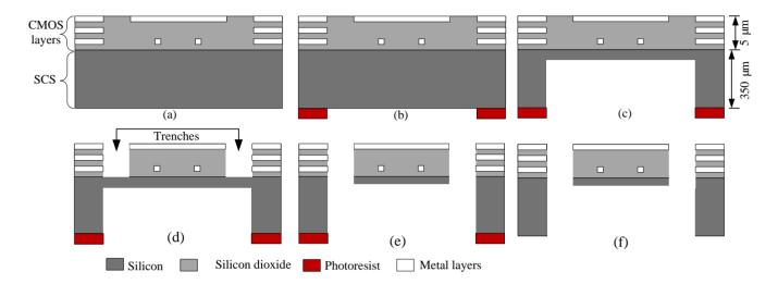
**Figure 2.** Schematic cross-sectional view of (a) Back grind; (b) PR layer deposited; (c) Anisotropic etching of Si from backside; (d) Anisotropic etching of SiO<sub>2</sub> from front side; (e) Isotropic etching of Si from front side; (f) Released device with photoresist mask removed.
