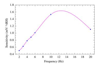
**Figure 11.** Sensitivity of the CMOS-MEMS humidity sensor *vs.* frequency.
