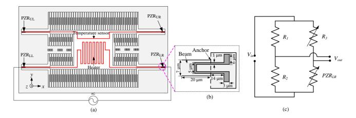
**Figure 3.** (a) Schematic of electrothermal actuation method and piezoresistive sensing; (b) A magnified view of PZR<sub>LR</sub>; (c) Wheatstone bridge circuit for measurement of the output signal.
