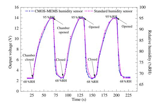
**Figure 12.** Response, recovery, and repeatability of the device and standard humidity sensor vs. time for three cycles at operating frequency of 2 Hz at 5 V<sub>pp</sub>.
