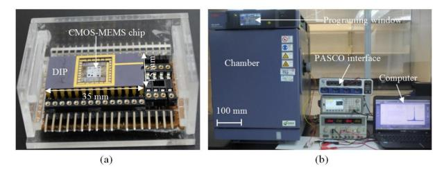
**Figure 4.** (a) Bonded and packaged device; (b) Experimental setup for measurement of the humidity response of the CMOS-MEMS device.
