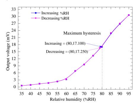
**Figure 7.** Output voltage vs. relative humidity at an operating temperature of 80 °C, corresponding to applied voltages of 6  $V_{pp}$  at a frequency of 4 Hz.
