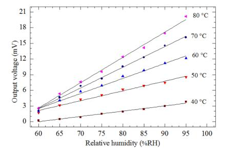
**Figure 9.** Output voltage vs. relative humidity at various applied voltages from 2  $V_{pp}$  to 6  $V_{pp}$  (corresponding to different operating temperatures from 40  $^{\circ}$ C to 80  $^{\circ}$ C) at a constant frequency of 2 Hz.
