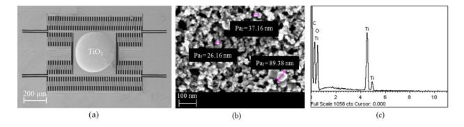
**Figure 6.** (a) FESEM image of CMOS-MEMS device with TiO<sub>2</sub> paste deposited on its plate; (b) Zoomed-in FESEM micrograph of TiO<sub>2</sub> nanoparticles. (c) EDX-spectrum of the TiO<sub>2</sub> on the plate.
