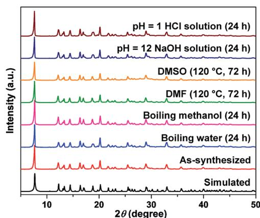
Fig. 2 PXRD patterns of as-synthesized CZU-1 and samples treated with aqueous solutions of HCl (pH = 1) and NaOH (pH = 12) for 24 h, hot DMSO and DMF solvent at  $120 \text{ }^\circ\text{C}$  for 72 h, and boiling methanol and water for 24 h.
