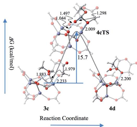
Fig. 6 The reaction profile of the deprotonation of  $\mu_4$ -OH for the termination of the ROP reaction process. Color scheme: O, red; H, light grey; C, gray; Zn, blue.
