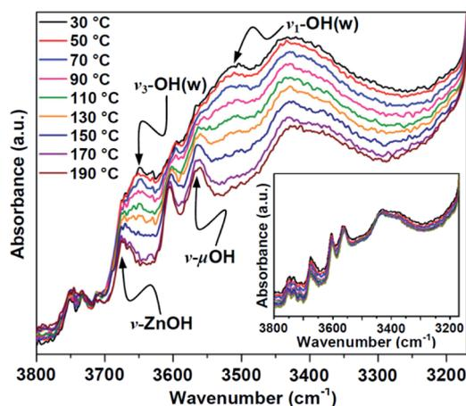
Fig. 7 Temperature-dependent *in situ* DRIFT spectra of as-prepared CZU-1 labeled with the changes in the stretching vibrations of the hydroxyl groups from 30 to 190 °C under a dry Ar atmosphere (the inset shows DRIFT spectra of activated CZU-1 samples showing the changes in the stretching vibrations of the hydroxyl groups upon decreasing the temperature from 190 to 50 °C).
