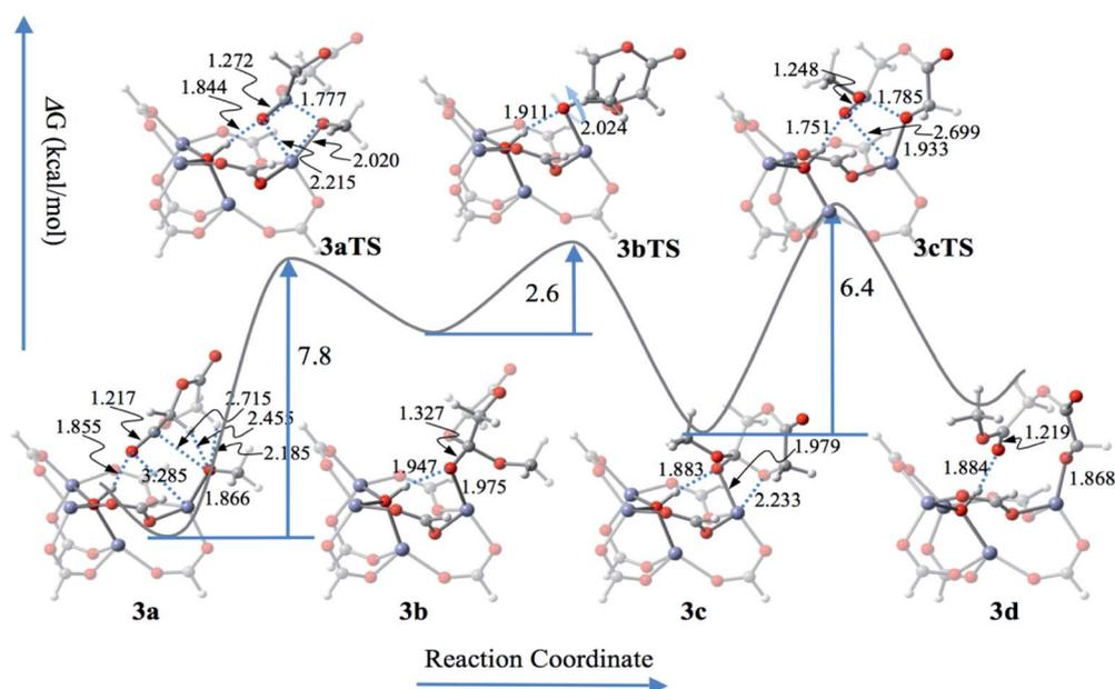
Fig. 5 The reaction profile of the ROP propagation process catalyzed by  $Zn_4(\mu_4-O)(COO)_6$ . Color scheme: O, red; H, light grey; C, gray; Zn, blue.
