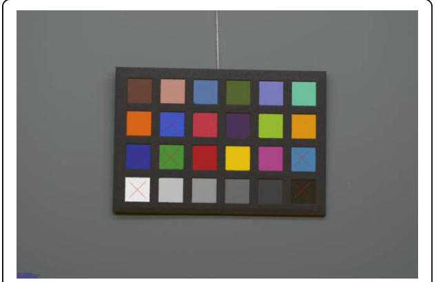
Figure 9 Example with Nikon D200: MBCC under illuminant D65 (6500 K). Camera: exposure bias -1, calibrated image.
