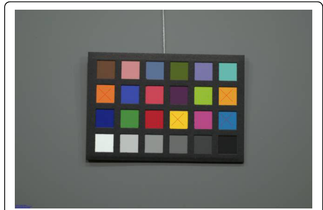
Figure 7 Example with Canon 10D: MBCC under illuminant A (3000 K). Camera: exposure bias -1, calibrated image.
