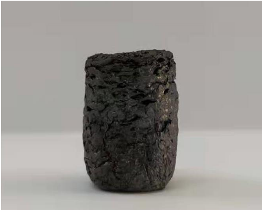
Figure S19. Related to Figure 3. Photograph of graphene foam.
