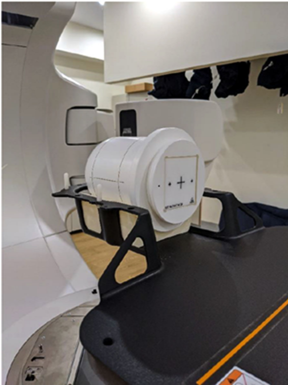
FIGURE 2 MultiMet-WL Cube inserted within the StereoPHAN, and positioned on the QFix Encompass SRS headboard. SRS, stereotactic radiosurgery; WL, Winston–Lutz
