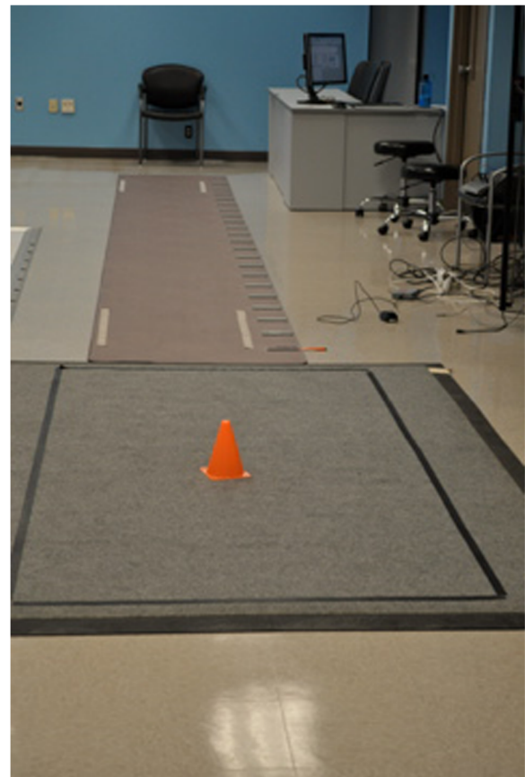
Fig. 1 Electronic Walkway Setup. The GaitRite electronic walkway is shown here, connected to the M 2 electronic walkway demonstrating the path patients took during study procedures to collect spatiotemporal parameters, including the turn task
