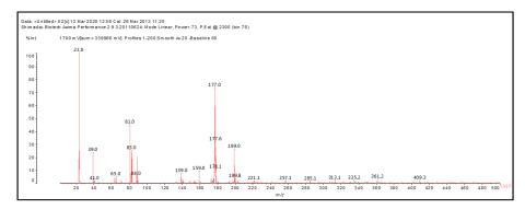
**Figure 4.** MALDI ToF spectrum of humins obtained at 180 °C from fructose, 20–500 Da range.
