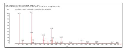
**Figure 1.** Matrix assisted laser desorption ionization time-of-flight spectrometry (MALDI ToF) spectrum of humins obtained at 180 °C from fructose, 20–500 Da range.
