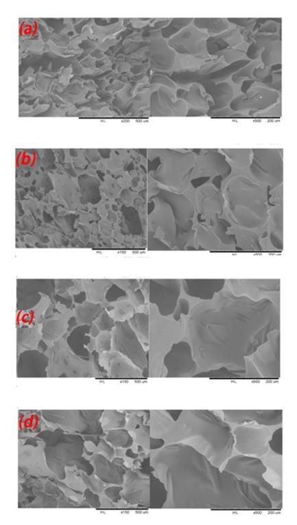
**Figure 10.** Effect on foam morphology of different proportions of humins. (a) F-H2.0-FA6-W1.5; (b) F-H3.7-FA6-W1.5; (c) F-H4.5-FA6-W1.5; (d) F-H5.9-FA6-W1.5.
