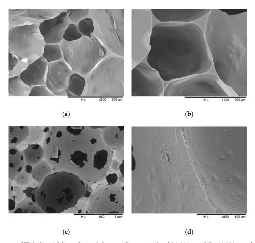
**Figure 7.** SEM of initial formulation 3 foam with magnitude of (a) 300× and (b) 10,000×, ambient temperature curing. SEM of initial formulation 4 with magnitude of (c) 80× and (d) 800×, 80 °C curing.
