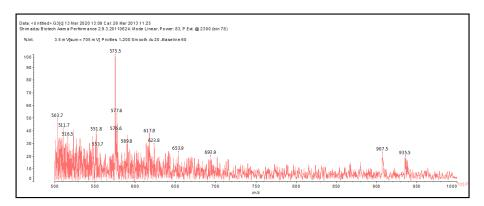
**Figure 3.** MALDI ToF spectrum of humins obtained at 150 °C from fructose, 500–1000 Da range.
