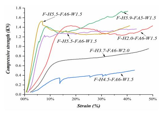
Figure 11. Compression strength as a function of percentage strain for the different tannin-humins foams.
