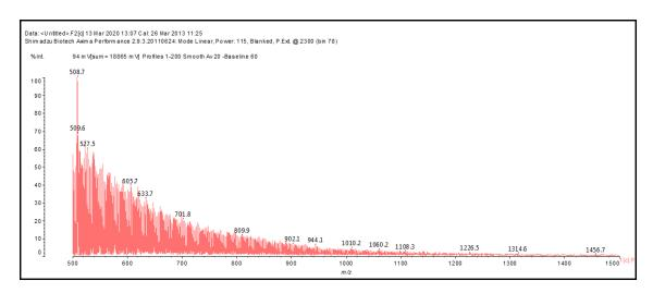
Figure 6. MALDI ToF spectrum of humins obtained at 180 °C from fructose, 500–1500 Da range.
