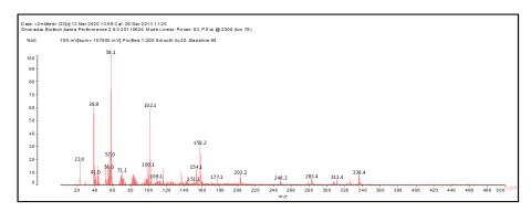
**Figure 2.** MALDI ToF spectrum of humins obtained at 150  $^{\circ}$ C from fructose, 20–500 Da range.
