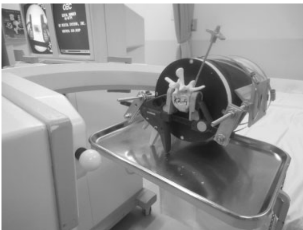
Fig. 4 Vertebra held in a stable position with the aid of a clamp installed on the C-arm.
