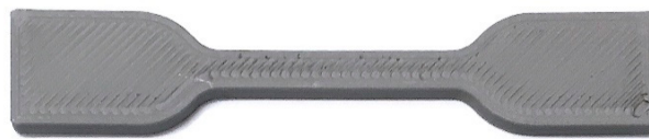
Figure 22. Specimen reprinted with optimized fused filament fabrication (FFF) parameters (extrusion temperature 260 °C, flow rate multiplier 130%, layer thickness 0.30 mm).
