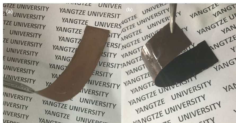
Figure 2. CuNW-based flexible composite substrate (a) and vulcanized substrate (b).
