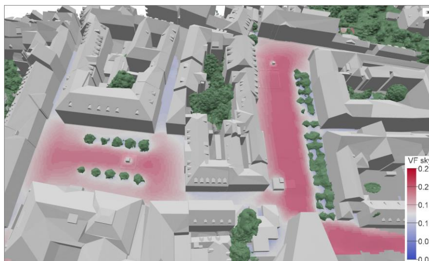
Figure A6. Spatially resolved evaluation of effective (physiologically-weighted) sky view factor (VF sky).
