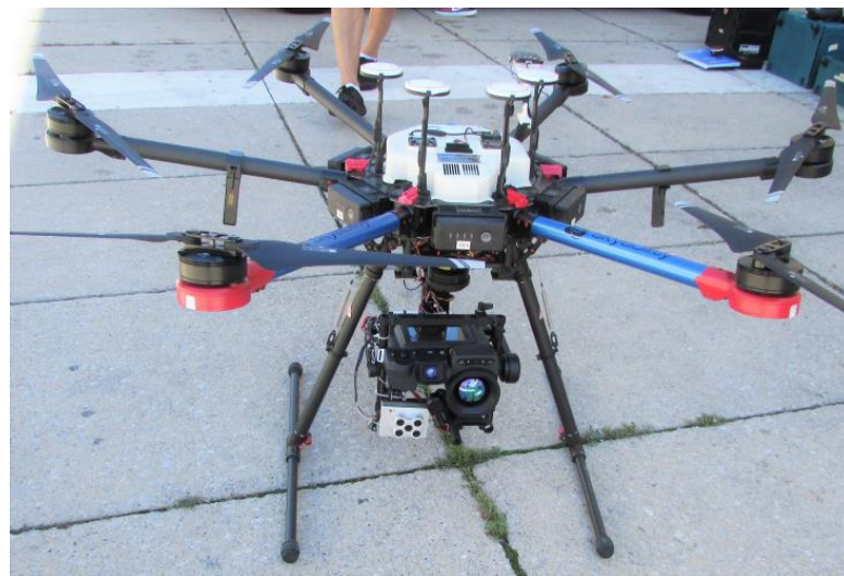
Figure 11. Drone Skyabilty M600 in the target area, with the IR camera (black) and multispectral camera (silver) on a gimbal system.
