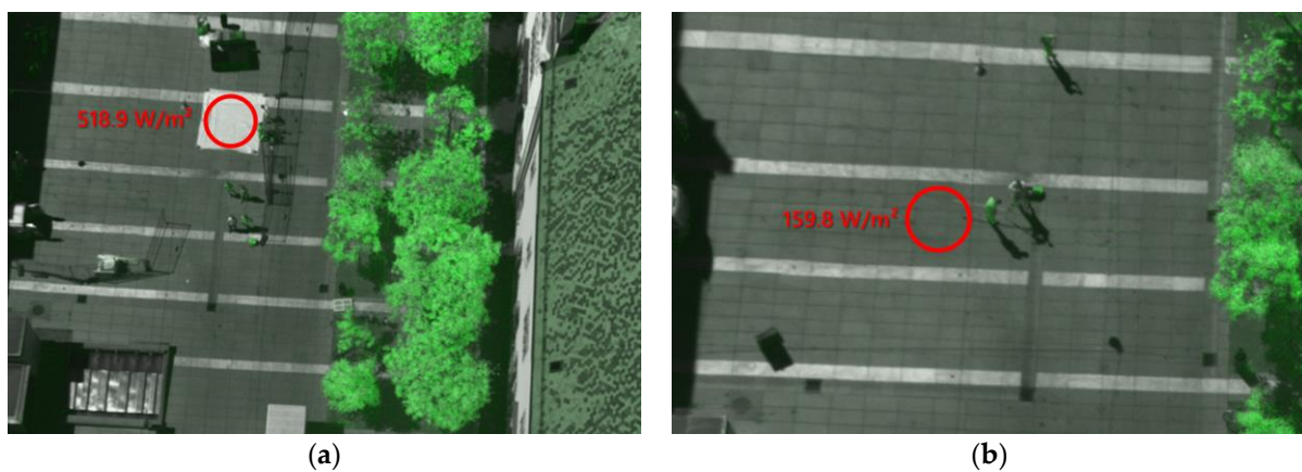
Figure 16. Images used for the validation of the shortwave radiant exitance detection and processing ((a): using a PP-fleece; (b): pavement).
