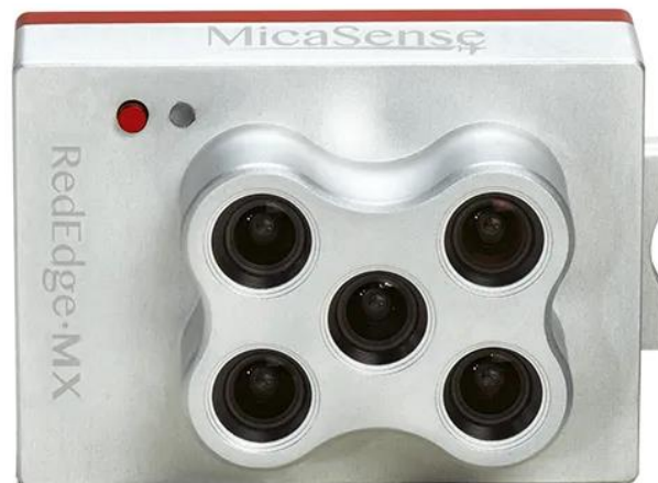
Figure 5. The multispectral camera used (MicaSense Red-Edge Mx).
