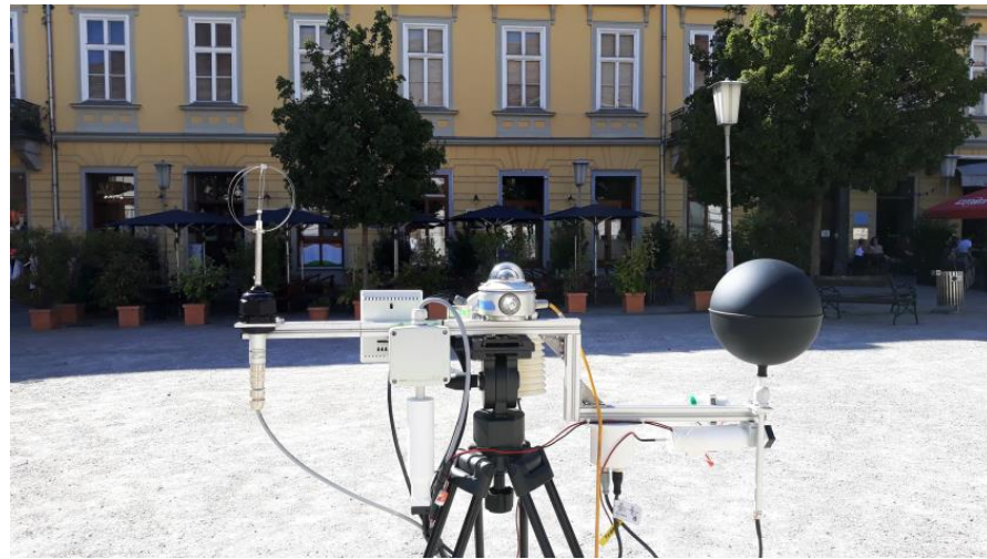
Figure 13. Spot measurement at location M5 (horizontally mounted pyranometer facing backwards).
