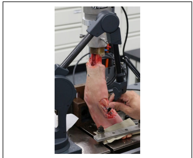
Figure 4. Making measurements with the 3D digitizer arm on the bone markers (screw heads).
