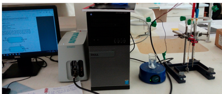
Figure 2. Cyclic voltammetry (CV) measurements were taken using Metrohm AutoLab PGSTAT 204 interfacing a computer with NOVA 2.0 as the control setup and operating software with set parameters.
