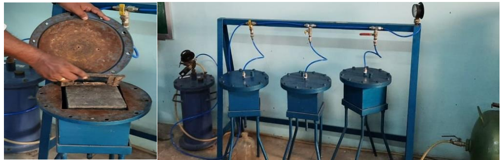
Figure 3. Water permeability apparatus and setup.
