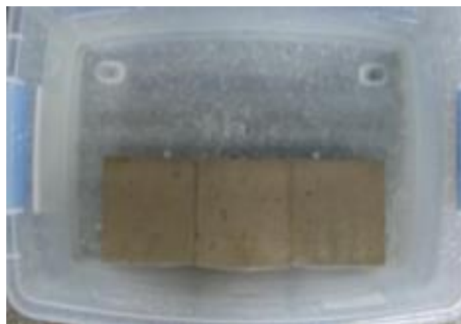
Figure 2. GPC specimens kept in sulfuric acid.
