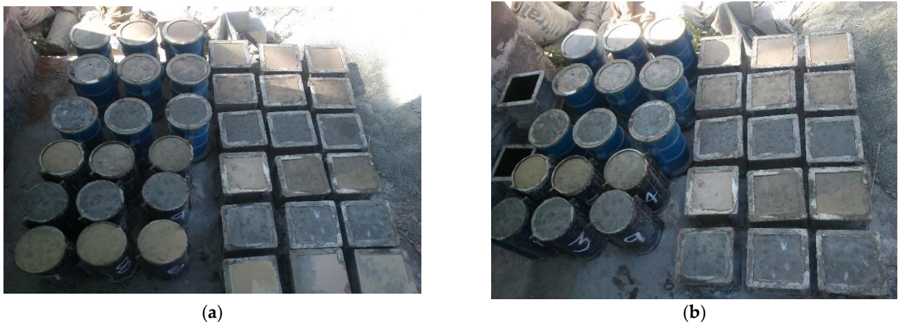
Figure 1. (a) GPC specimens, (b) CC specimens.
