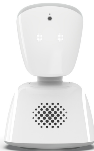
Figure 1 AV1: a robot for children who cannot attend school because of long-term illness (photo: No Isolation).
