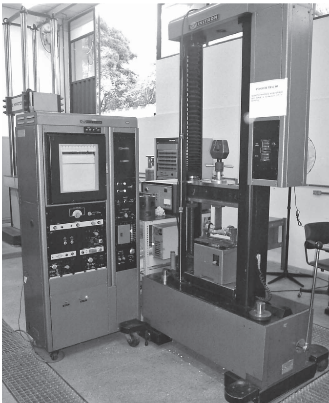
Figure 2 – Instron TTDML® universal test machine (Canton, MA, USA). Mechanical test laboratory of the Nuclear Technology Development Center of the National Nuclear Energy Commission (CDTN/CNEN)
