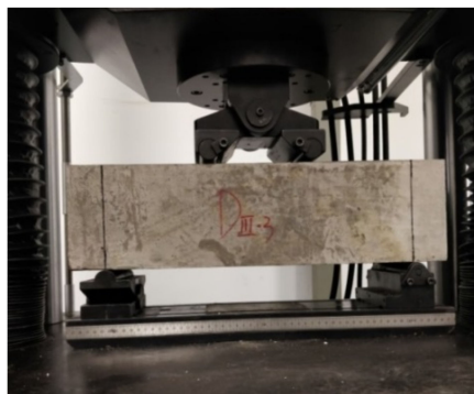
Figure 6. The four-point bending strength test.
