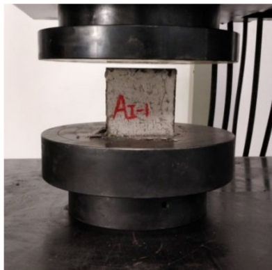
Figure 5. The compressive strength test.
