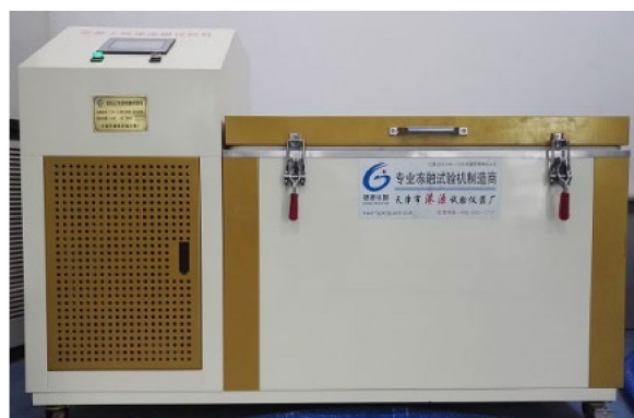
Figure 3. The rapid cyclic freeze–thaw tester.
