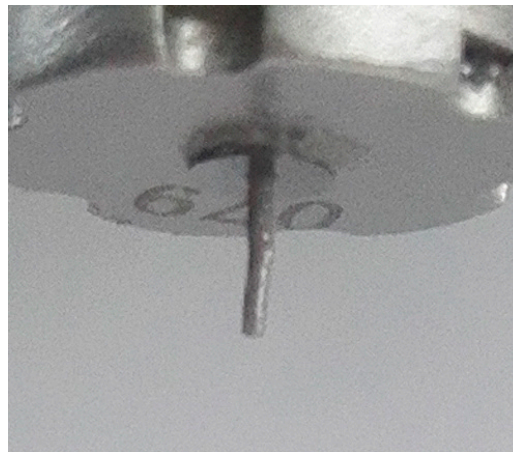
Figure 10. Solder paste suspension at the nozzle.
