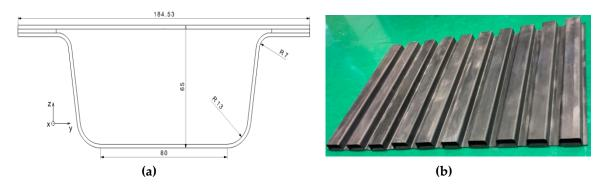
**Figure 2.** Rocker panel component in carbon fiber. (a) Cross section of the rocker panel. (b) Test specimens.
