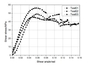
Figure 1. Shear stress vs. shear angle curve.
