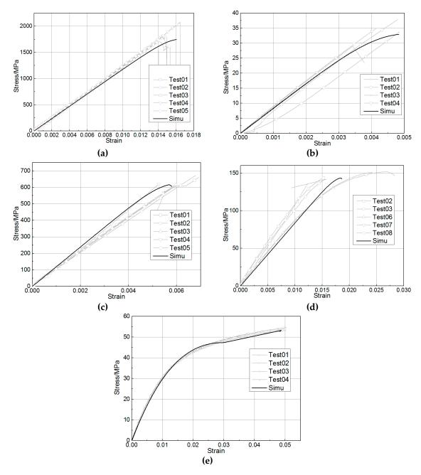
**Figure 5.** Comparison between test and simulation at the coupon level. (a)  $0^{\circ}$  tension. (b)  $90^{\circ}$  tension. (c)  $0^{\circ}$  compression. (d)  $90^{\circ}$  compression. (e) Shear.
