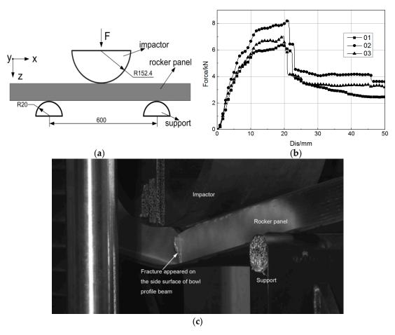
**Figure 3.** Three-point bending test. (a) Three-point test diagram. (b) Force-displacement curve. (c) Onset of fracture.
