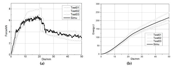
**Figure 6.** Comparison between test and simulation at the component level. (a) Force–displacement curve. (b) Energy absorption–displacement curve
