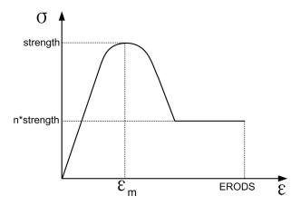
Figure 4. Shear stress vs. shear angle curve.
