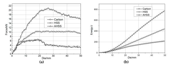
**Figure 7.** Three-point bending simulation results of steel and carbon fiber. (a) Force–displacement curve. (b) Energy absorption–displacement curve.
