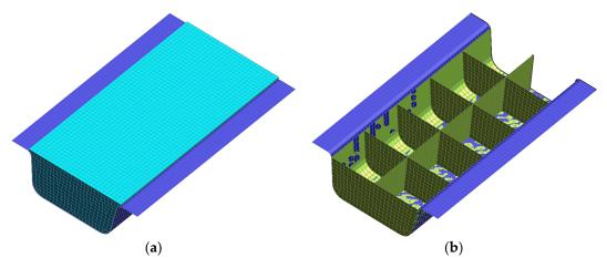
Figure 8. Reinforcement approaches. (a) Foam core filling. (b) Polypropylene reinforcement.
