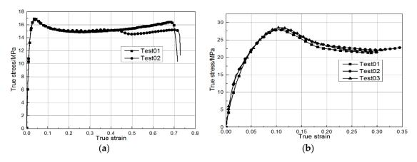
Figure 9. True stress–true strain curves of polypropylene material. (a) Tension. (b) Compression.
