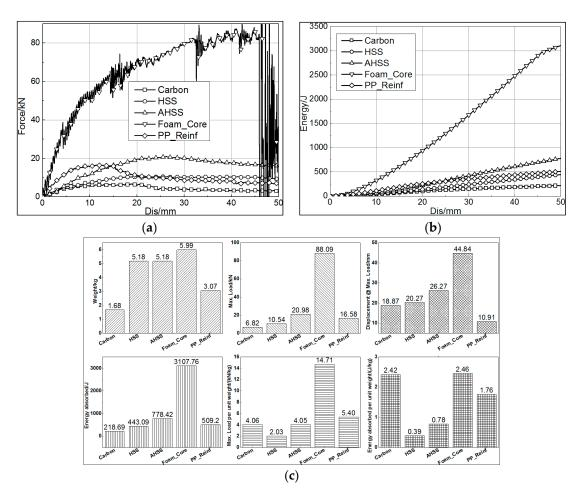
**Figure 10.** Comparison of the performance of different rocker panel components. (a) Force–displacement curve. (b) Energy absorption–displacement curve. (c) Histograms of parameters showing the bending performance of the rocker panels.
