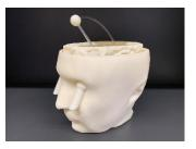
**Figure 4.** Upside down head phantom including the complex brain and an extra cavity as a muscle container. The stroke and the connected pipes are designed in a way to pass through the cylinders which are connected to the brain cavity and can be fixed in a random location inside of it.
