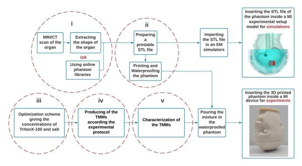
Figure 1. Three-dimension (3D) Printed benchmark phantom flowchart for microwave imaging.
