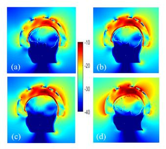
**Figure 7.** Normalized electric field magnitude distribution inside and outside the head including cavities made of: ABS shell (**a**), without ABS for stroke (**b**), stroke and brain (**c**) and only bone (**d**).
