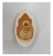
Figure 3. Upside-down configuration of the head phantom including the simple brain cavity.
