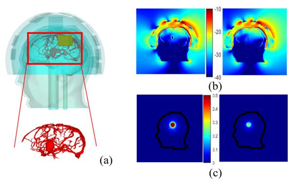
**Figure 9.** Head phantom including brain vessels and an elliptical stroke inside (**a**). Normalized magnitude of the E-field inside and outside the head by taking blood vessels into account and the elliptical stroke, surrounded by ABS (**b**, left), with no ABS (**b**, right); the corresponding differential E-field (**c**, left) and (**c**, right) respectively.
