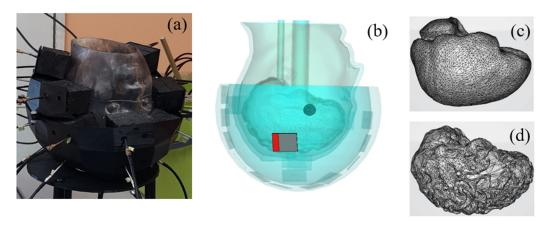
**Figure 5.** The imaging system [5], including a head phantom with a stroke mimicking anomaly and a 24-antenna array conformal to the head (**a**,**b**). Two different models of the brain are used: a simple (**c**) and a complex with convolutions (**d**).
