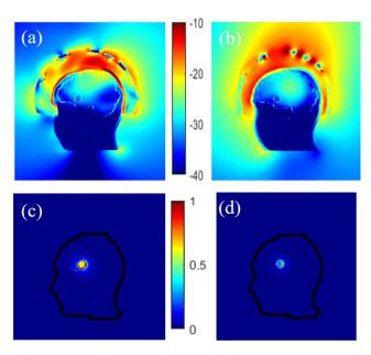
**Figure 6.** Normalized electric field magnitude distribution inside and outside the head for 2 different coupling mediums, TX-100/salted water (a) and air (b). The corresponding differential field distribution, TX-100/salted water (c) and air (d) respectively.
