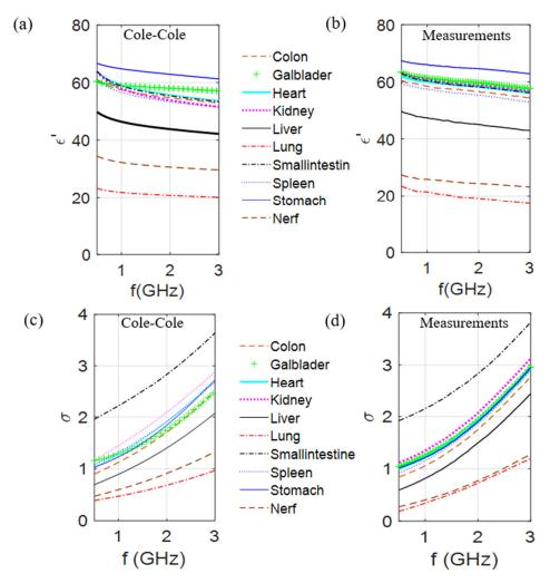
**Figure 2.** Comparison of the dielectric constant and conductivity of 10 different biological tissues of the values obtained from the Cole–Cole model (**a**,**c**) with the measured values (**b**,**d**) of produced mixtures at room temperature, over the [500 MHz to 3 GHz] frequency range.
