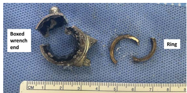
Fig. 2. The boxed wrench end and ring after destructive removal.
