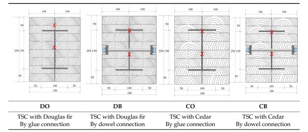
Table 1. Cross-section of timber-steel composite (TSC) specimens.
