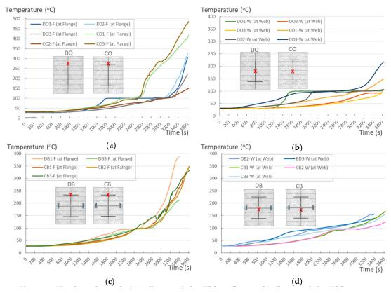
**Figure 14.** The thermal record of (**a**) all types of glue TSCs at flanges; (**b**) all types of glue TSCs at webs; (**c**) all types of dowel TSCs at flanges; and (**d**) all types of glue TSCs at webs.
