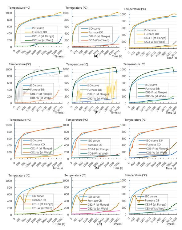
**Figure 11.** Specimen heating temperatures. (a) Douglas fir TSC assembled using glue; (b) Douglas fir TSC assembled using dowels; (c) cedar TSC assembled using glue; (d) cedar TSC assembled using dowels.
