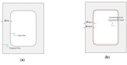
**Figure 2.** Concept for charring models. (a) Actual char depth (CD)  $d_{char}$ ; (b) CD  $d_{char,0}$  for one-dimensional charring and notional charring depth  $d_{char,n}$ .
