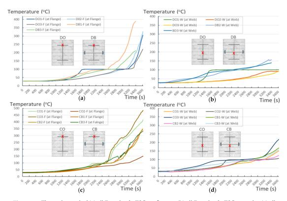
**Figure 13.** Thermal record of (a) all Douglas fir TSCs at flanges; (b) all Douglas fir TSCs at webs; (c) all cedar TSCs at flanges; and (d) all cedar TSCs at webs.
