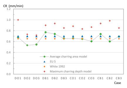
Figure 12. Experimental results and comparison of CR models.
