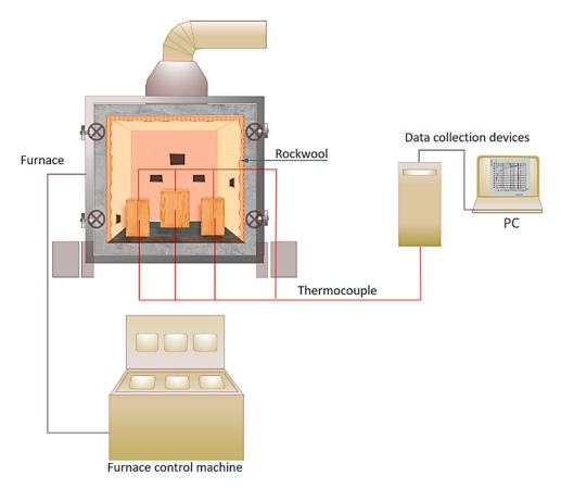
Figure 6. Furnace and test setup.
