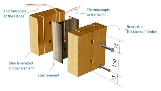
Figure 4. TSC specimen with dowel connection equipped with thermocouples (unit: mm).
