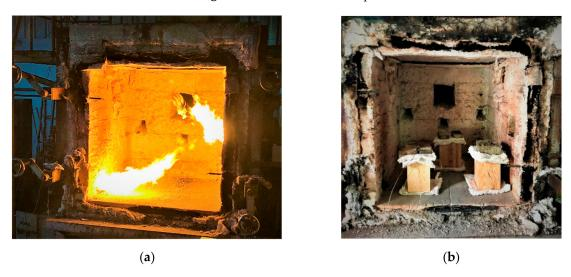
Figure 7. (a) location of fire; (b) arrangement of test specimens.
